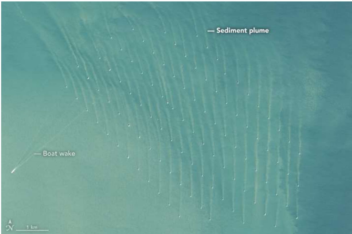
Figure 5 - Satellite Image from Thanet offshore wind farm showing the suspended sediment plumes from each monopile.
